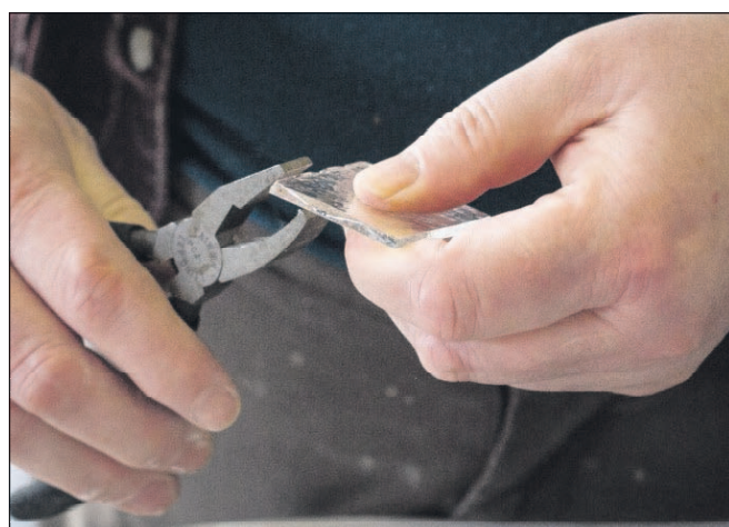
Jamie Boyd cuts a segment of glass used in creating the glass tiles. Joshua Bessex/The Daily Astorian
