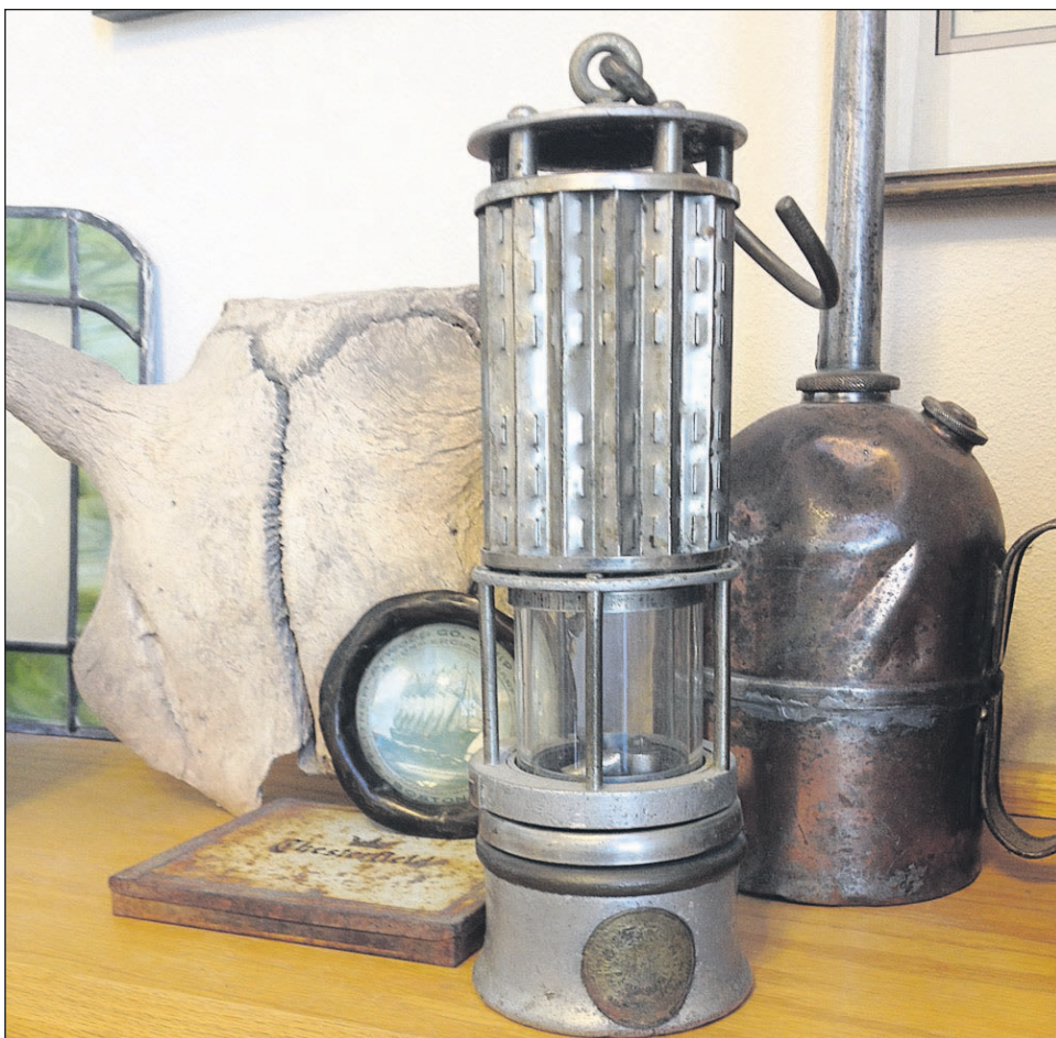
In 1830, safety lamps, like the one pictured here, were considered one of the greatest lifesaving inventions of the modern era, allowing miners to carry open flames for illumination in underground coal workings without setting off methane explosions. It is pictured with a bison skull and a few other objects in Matt Winters' "cabinet of curiosities."
