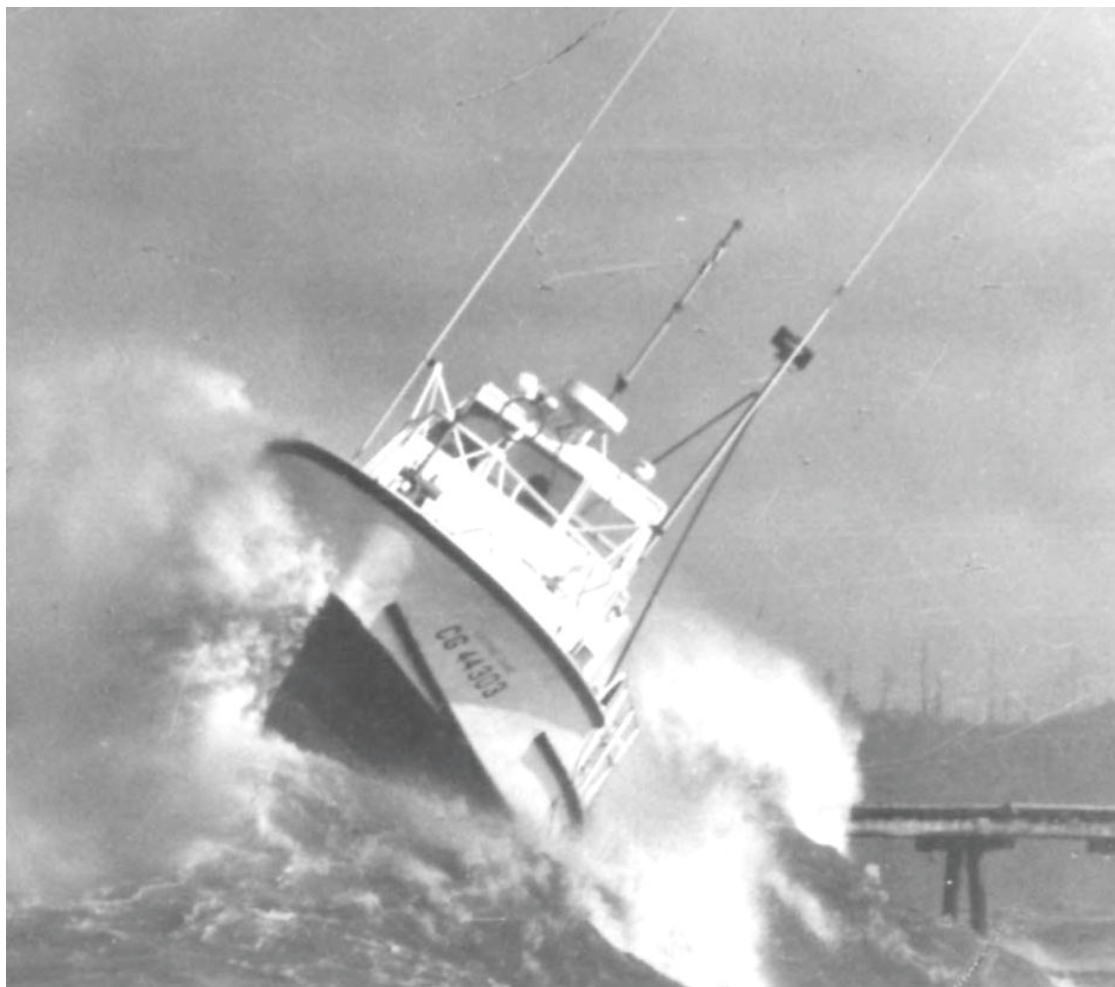
44-foot motor lifeboat: Self-righting and self-bailing; probably capable of surviving far more severe conditions than what it was rated for (30 foot seas, 50 knots of wind, 50 nautical miles offshore, 20 foot breaking surf and a 125 towing capacity).
