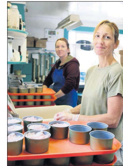
Christie Bartlett, right, and Kim Pickering pack fresh tuna into cans at the Sportsmen's Cannery in Seaview, Washington. Each can is packed by hand, individually weighed, then sealed and processed in one of the facility's twin pressure cookers, which have been in use since the 1950s.
