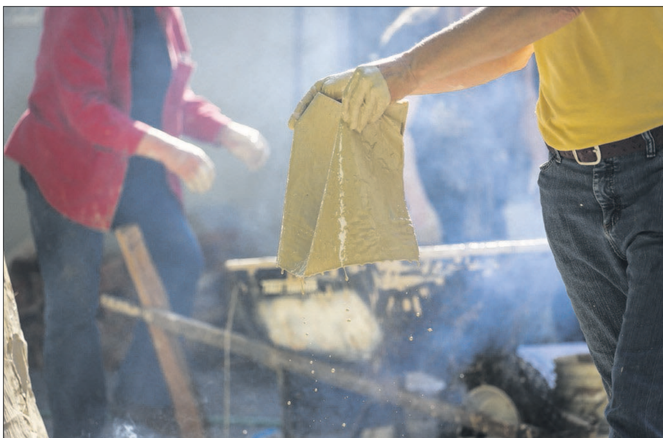
The outside of the paper kiln was coated with layers of newspaper dunked in clay and water. Due to the high heat inside the paper kiln, it had to be constantly maintained with new paper throughout the day and night.
