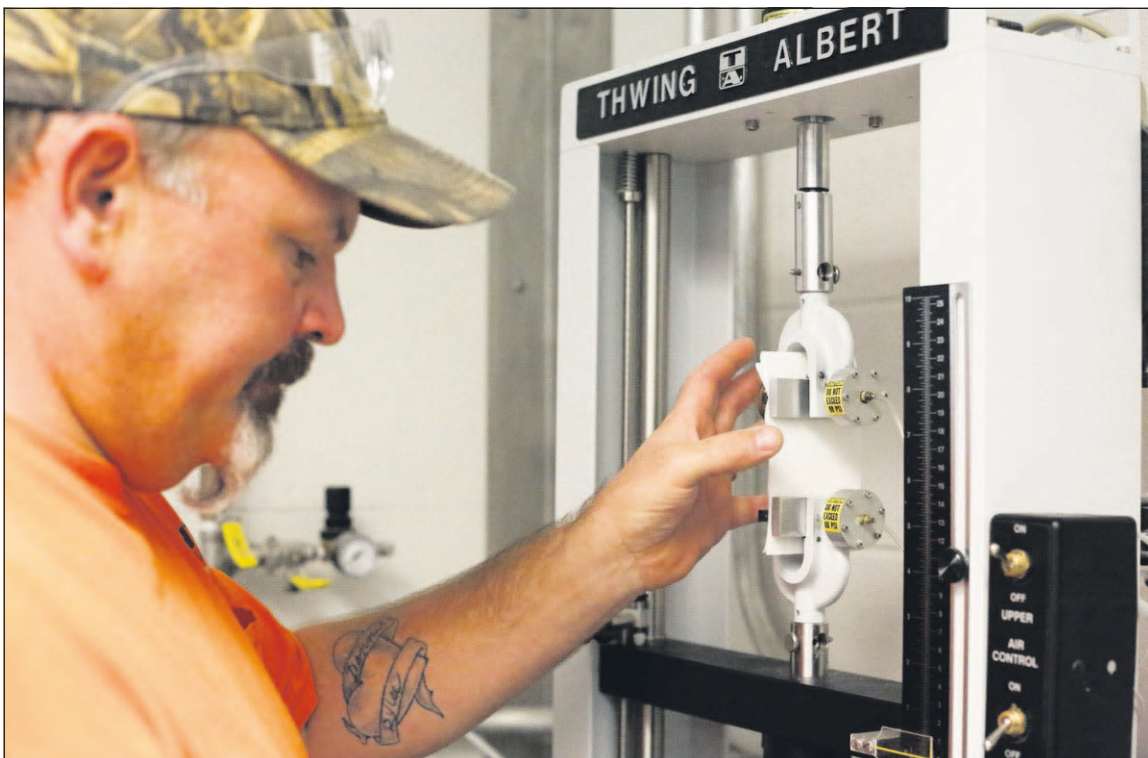
Jim O'Brien tests the tensile strength of samples of Brawny paper towels. The strength is measured both while the paper towels are dry and wet. The samples are also tested for absorbency.
