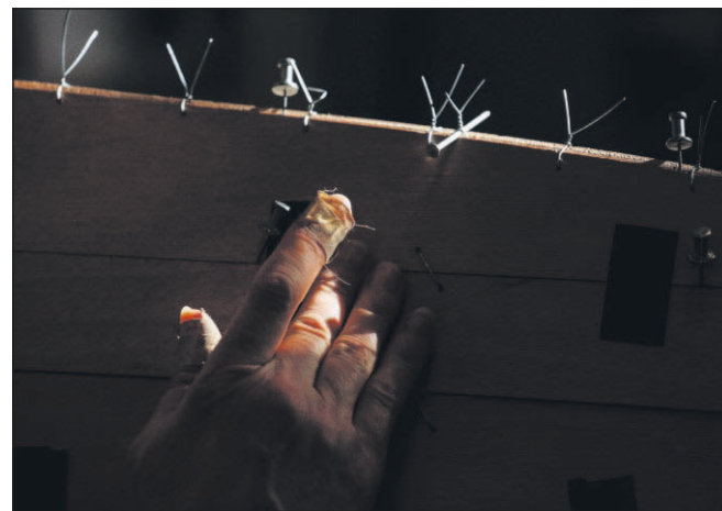
JOSHUA BESSEX — The Daily Astorian Amy Hatton runs her fingers along the hull of her kayak during a session Tuesday. In order to keep the panels of the hull smooth, builders used tape, wire stitches and push pins.
