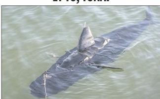
Another dorsal-finned critter is roaming the ocean, but this one is man-made: The GhostSwimmer roboshark, pictured in a U.S. Navy photo, a shark-shaped underwater robot that is the Navy's latest toy to gather data and videos on tides, currents and weather, according to a story on Gizmag.com (http://tinyurl.com/roboshrk). Both its body shape and swinging tail mimic its namesake.
