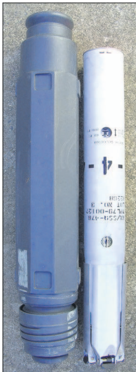
Peter Ellis via en.wikipedia The AN/SSQ-47B is an 'active' (pinger) or ranger (range measuring) sonar sonobuoy.
