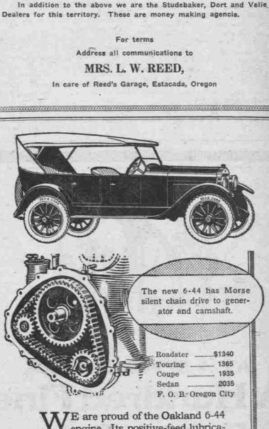
engine. Its positive-feed lubrication, its overhead valves, its "honed" cylinders, its special pistons and rings, its adjustable silent chain drive to cam shaft, its special bronze-back main bearings are just a few of the expensive construction features.
