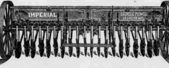
Enlarged view of Foot-Board, Horse-Lift and Hand Levers. The inner levers with turned in handles are horse-lift levers. The outer levers shown as broken off are hand-lift levers used to put on pressure, or to lift discs when drill is standing.
