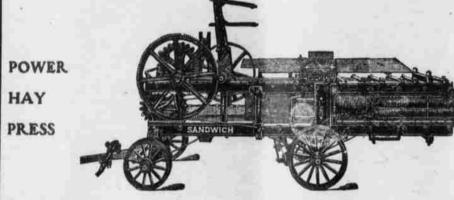
Simple, Strong, Compact; can be operated to full capacity with an 8-horse-power Stover Engine. Self feeder. Handles large feed with great accurateness. Block dropper absolutely safe and sure. Slow, steady Speed-No quick jerky motions to ruin press and nerves of operator. Long plunger arm uncovers large feed opening. No superlative cogs and gears.—A BUSINESS OUTFIT FOR BUSINESS MEN.
