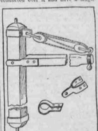
DETAIL OF DERRICK. tree attached for a horse when it is necessary to lift a more than ordinary heavy object from the cellarway.
