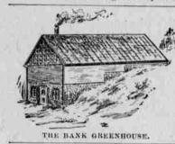
rough field stones. The entrance is at the further end, steps down from the doorway to the greenhouse floor being provided. Such a building will be exceedingly warm in winter, not only because of the earth bank, but because heat can be generated and sent to a floor above much more readily than it can be generated upon and diffused over a single floor.-American Agriculturist.
