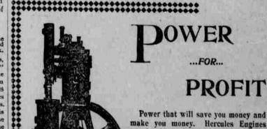
make you money. Hercules Engines are the cheapest power known. Burn Gasoline or Distillate Oil; no smoke, fire, or dirt. For pumping, running dairy or farm machinery, they have no equal. Automatic in action, perfectly safe and reliable. Send for illustrated catalog.
