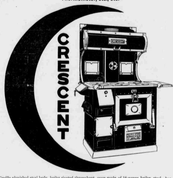
A one-piece Wellsville planished steel body, boiler riveted throughout, oven made of 16-gauge boiler steel, has duplex grates for wood and coal, cast-iron flare back, also cast extension firebox for long wood; heavy asbestos-lined walls; is as well constructed as any range sold, regardless of price. You don't have to take our word for it—come and see, it's to your interest, for naturally you want the best range to be had for your money.
