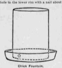
five-eighths of an inch from the bottom; fill with water and place a dish over same (diameter of dish must be about two inches larger than diameter of can).
