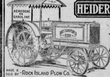
7 speeds forward and 7 reverse is just one of the features made possible by the Heider Patented Friction Transmission. It means less gears, less expense, smoother power, steadier power and ease of operation.
