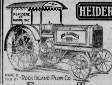
7 speeds forward and 7 reverse is just one of the features made possible by the Heider Patented Friction Transmission. It means less gears, less expense, smoother power, steadier power and ease of opera-
