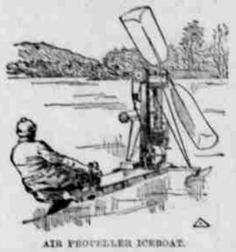
AIR PROPELLER ICEBOAT. blades are four feet long, with a ten foot swing, and are driven by a four horsepower motor. The speed is only ten miles an hour on fair ice, partially due to the fact that the machine weighs 150 pounds more than is necessary and about one horsepower is lost in chain play.
