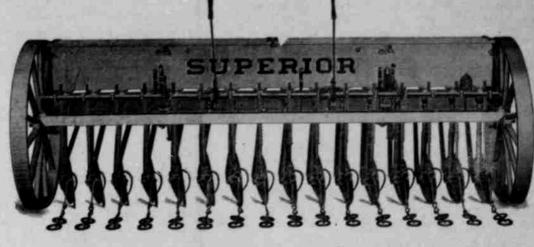
Consisting of 10-7, 12-7, 14-7 and 16-7, all right-hand Single Disks, with or without grass seed attachments. The effective feed method of lubricating the discs, style of discs and other good points all combine to make the SUPERIOR the best Seed Drill made.
