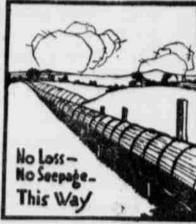
1-The lumebr used in making American quality wood pipe is of best grade Washington yellow fir and is free from flaws. It is thoroughly seasoned by kiln drying, which makes it strong and durable.
