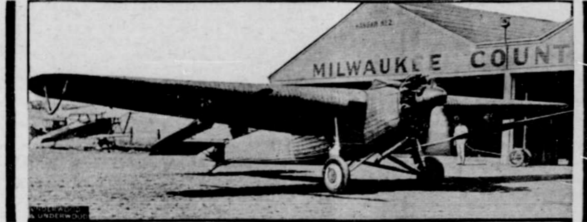
The "Maiden Milwaukee," all-metal monoplane which has been purchased from the Hamilton Metalplane company of Milwaukee by the Johnson Aeroplane company of Delray, Fla. Jesse C. Johnson has converted the plane into an experimental helicopter...
