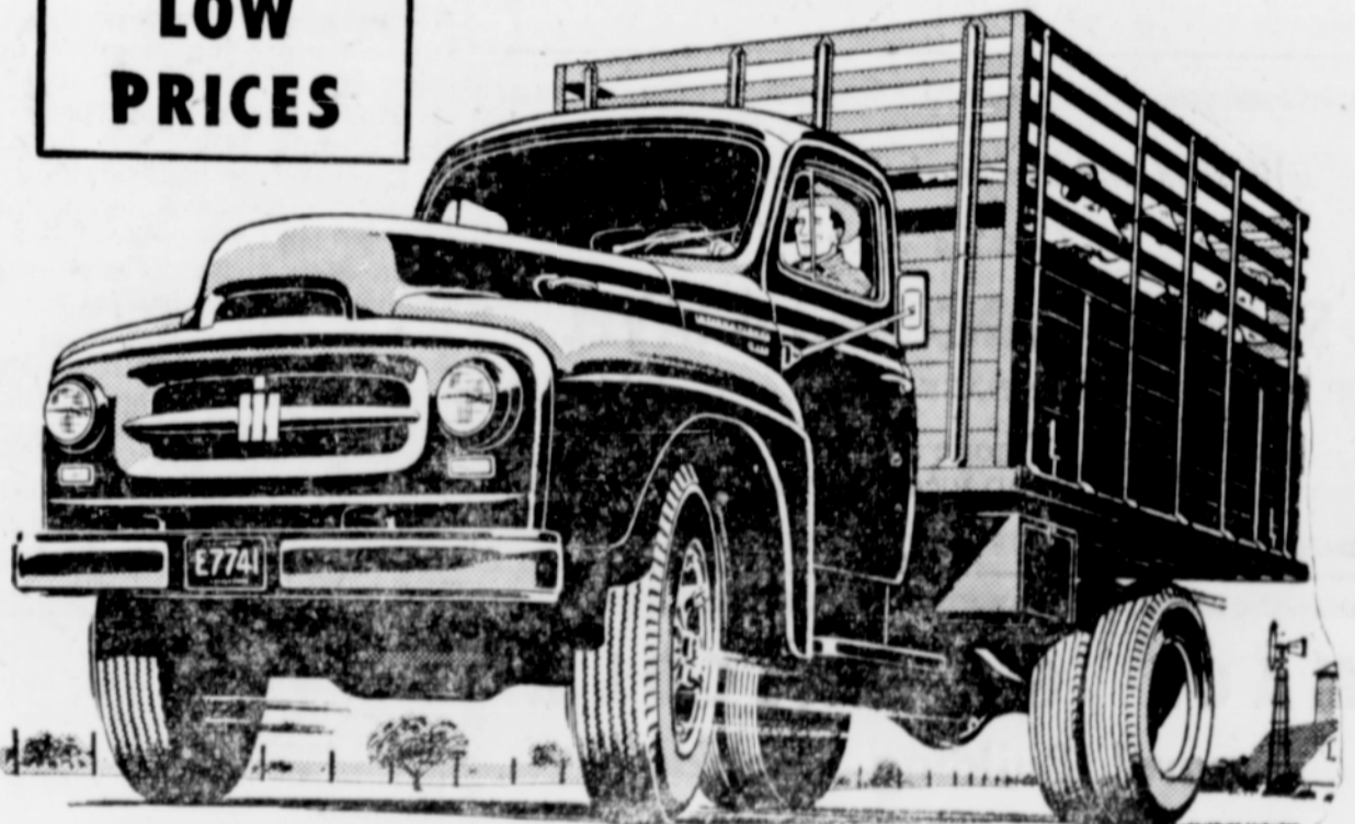
International Model R-160 with combination body. R-160 Series, GVW ratings, 14,000 to 17,000 lbs.
