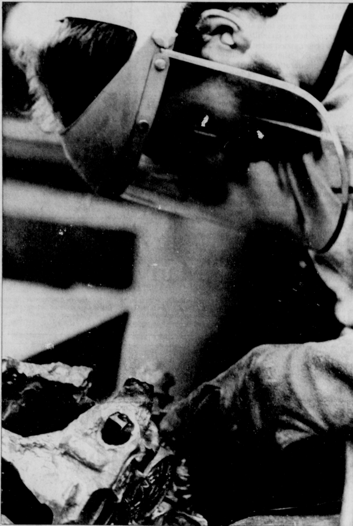
Brad Lorang grinds a piece after it has been cast to eliminate imperfections and bring it closer to the artist's original.
