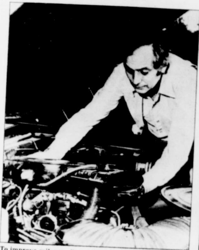
To improve mileage, first remove air cleaner, then squirt cleaner directly into carbureator.
