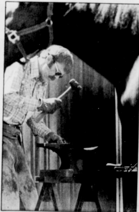
Most shoes are pounded into shape while they are cold, then thrust into hot coals to open up the nail holes again.
