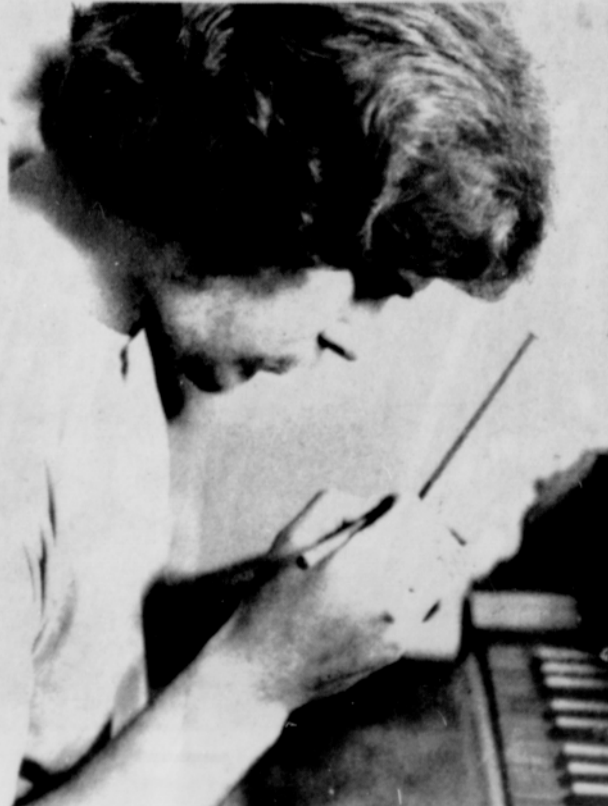
QUILL FILING is part of regular maintenance on a wooden harpsichord, an instrument that plucks the keys rather than strike them like the piano.
