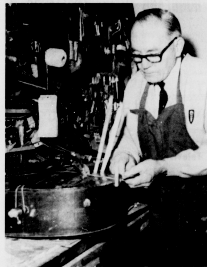
BATTERED INSTRUMENT gets a facelift from Frank H. Busch, who has been an accredited violin maker for 54 years. Busch said he likes a challenge as he fitted a replacement piece on the instrument.
