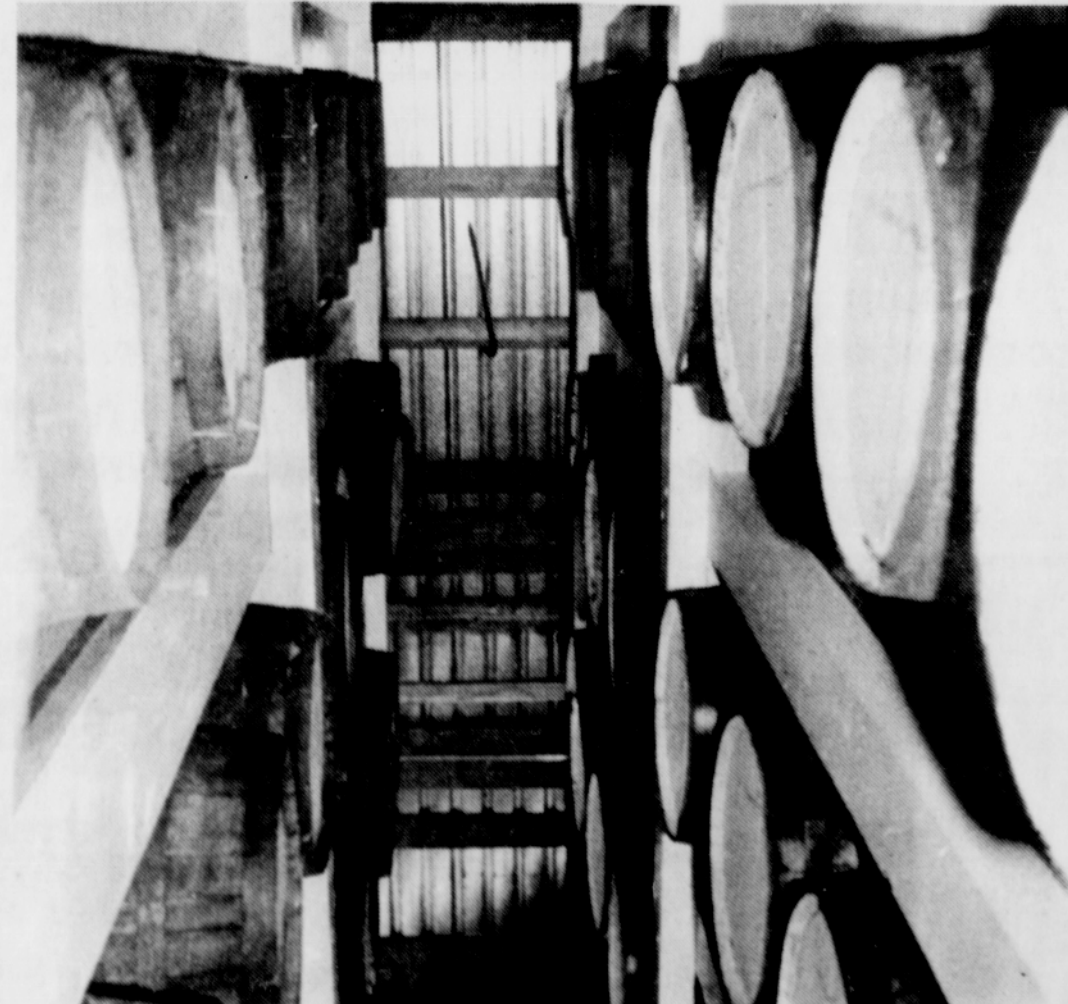
ROWS AND ROWS of 50 gallon oak barrels are used to store and age the several different natural fruit juices. Water seals in the top of each barrel allow gases to be
