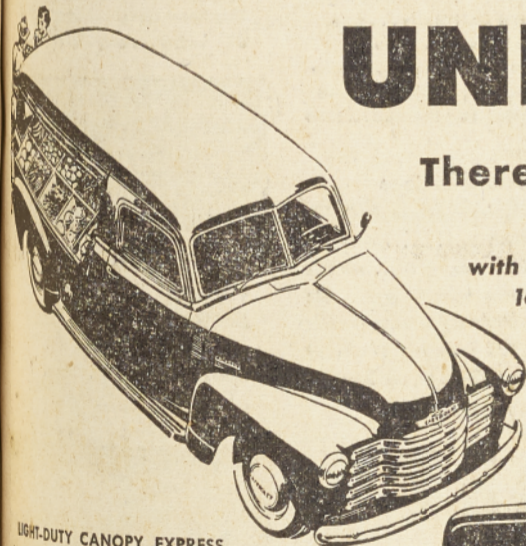
LIGHT-DUTY CANOPY EXPRESS Model 3107—116-inch wheelbase, Maximum G.V.W. 4600 lbs. Also available in Medium-Duty Model 3807—137-inch wheelbase, Maximum G.V.W. 6700 lbs.
