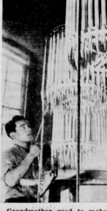
Grandmother used to make her bayberry candles in a copper pot, one at a time. Now, in a Philadelphia, Pa., plant, great bunches of wicks are dipped simultaneously until they are the desired thickness. The candles, made from berry wax, give off a distinctive aroma—the incense of Christmas.
