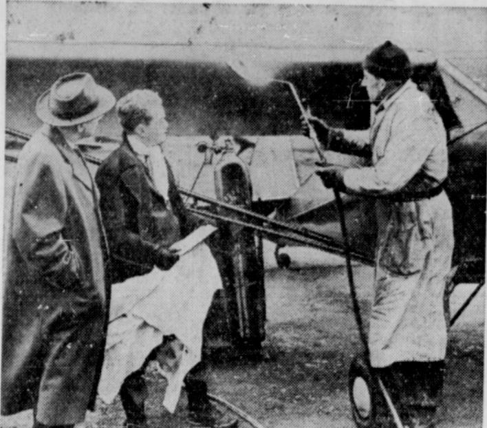
A mechanic using a blow torch demonstrates how the wings of a light plane have been rendered fireproof with a covering of woven fabric which replaces ordinary cotton or linen fabric. The glass fabric has the added advantage of being non-shrinkable, non-stretching and rot-proof.
