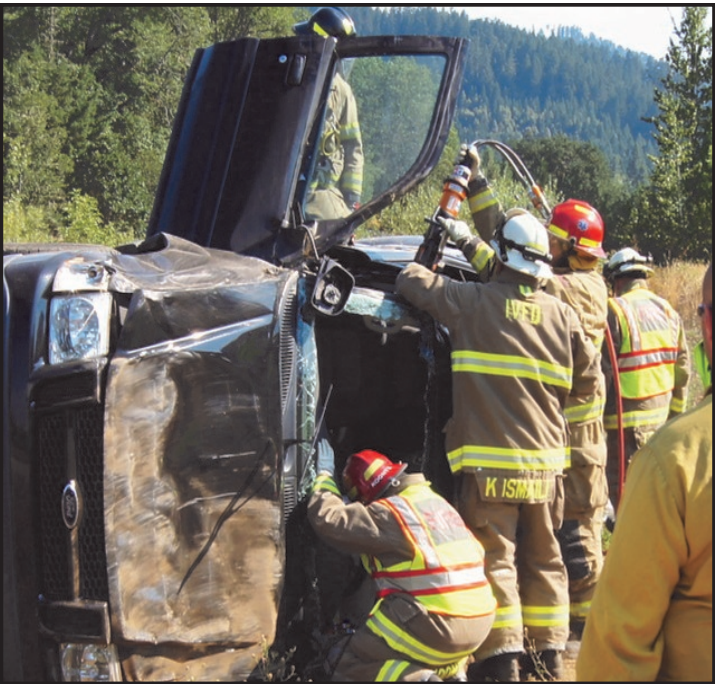
IVFD Responded to a Rollover Traffic Accident on Takilma Rd. Above—volunteer Captain Tom Zulliger uses hydraulic cutters to remove the vehicle's roof.
