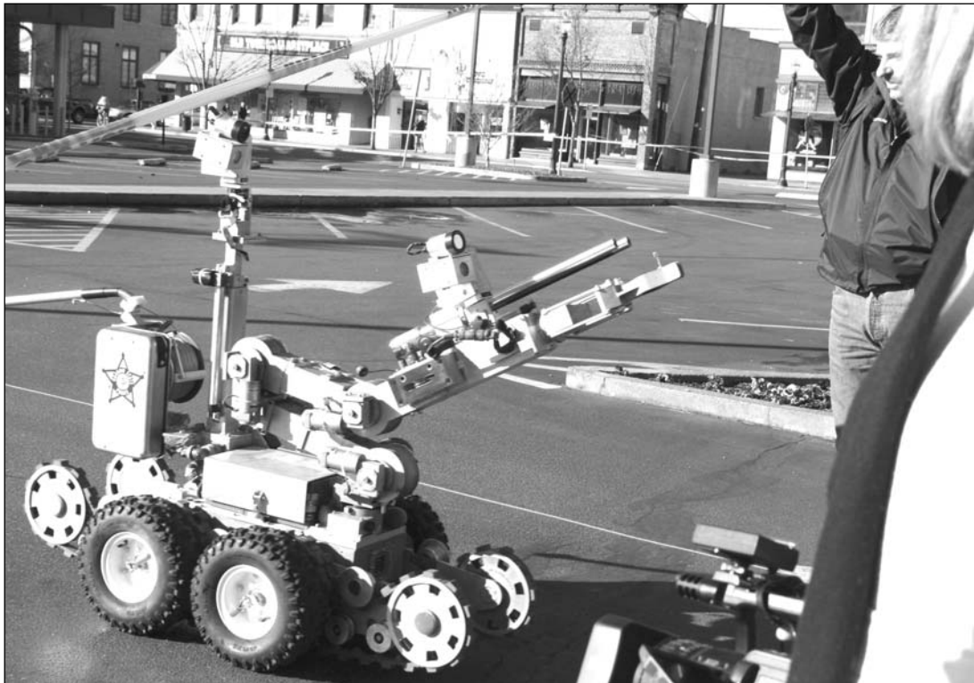
This tethered Oregon State Police robot, equipped with video camera and a water cannon, was deployed to investigate the 'bomb'. (Photo by Michelle Binker, Illinois Valley News )
