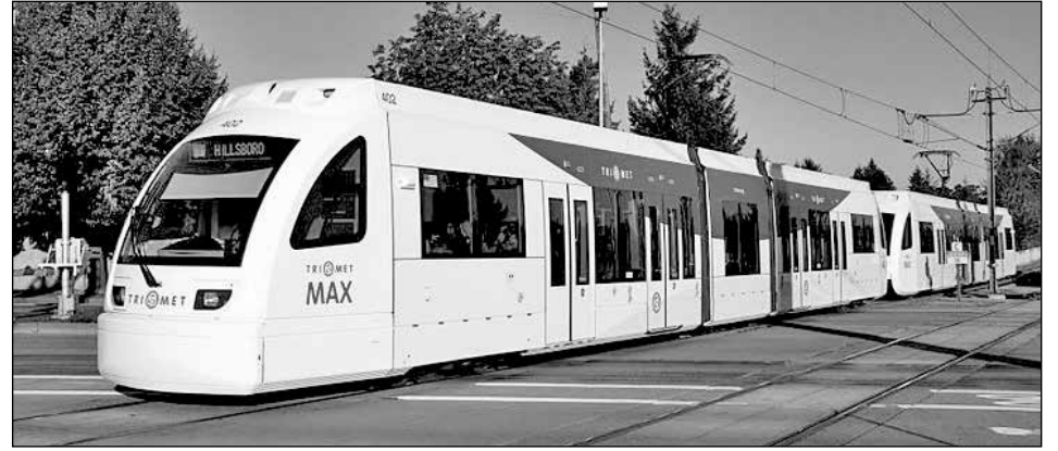
A MAX light rail train with Type 4 cars crossing 185th Avenue from Beaverton into Hillsboro. (Photo by Steve Morgan, Wikimedia creative commons license)
