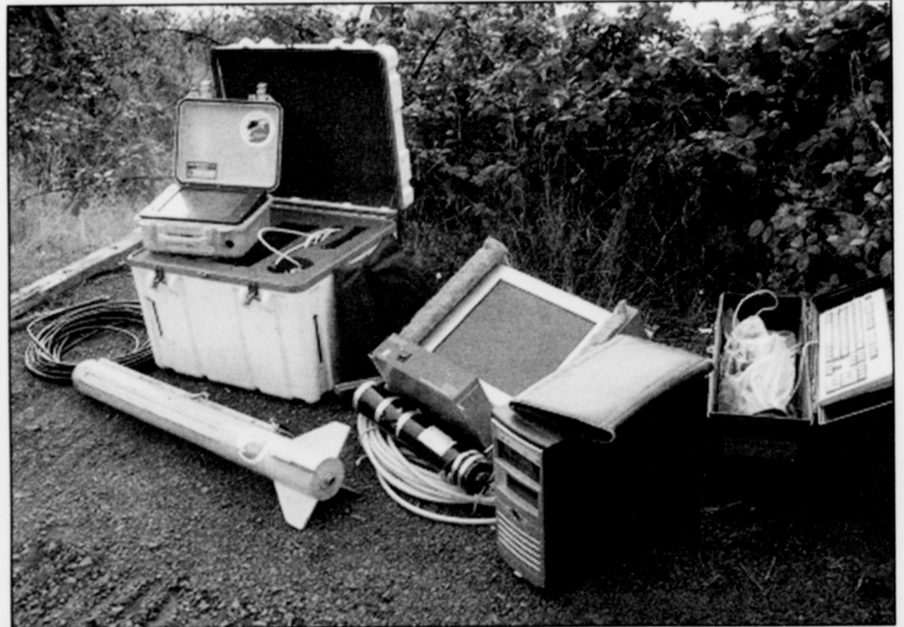
Sonar and computer equipment are used to locate underwater logs (crane monitor in center).
