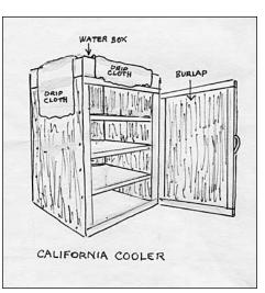
was built into the house by leaving an opening in the floor and ceiling, then building a cabinet or closet over the openings. This allowed the cool air from under the house to circulate into the space. A screen was placed over the openings to
