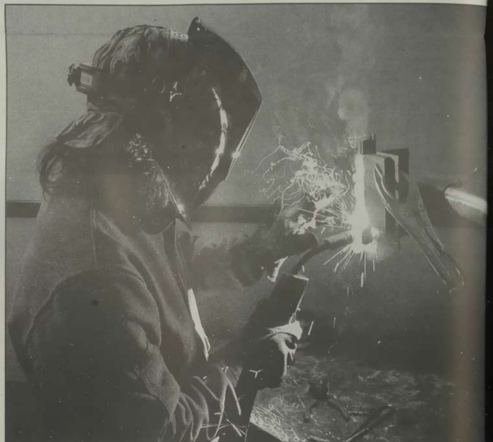
Welder Vince Priest operates a gas metal arc-welder as he works toward certification to earn more in his chosen profession. Brad Heineke Clackamas
