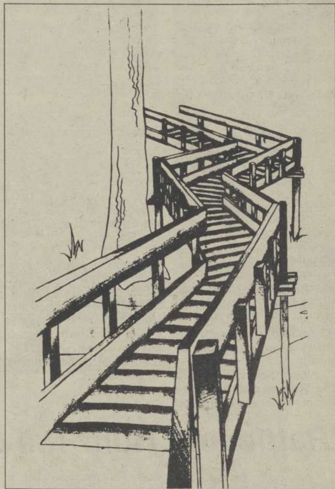
This bridge is just one example of the uses of plastic lumber. Another use for it would be in the construction of signs for the Environmental Learning Center. Plastic lumber is produced from waste plastics, such as milk jugs and soda pop containers.
