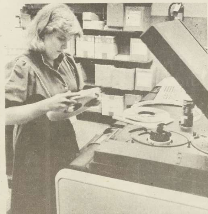
A BRAIN BREAK. Operator Robin Sharpe changes memory in the new computer system. The procedure is repeated twice a day to avoid losing information due to power failure. Fobert
