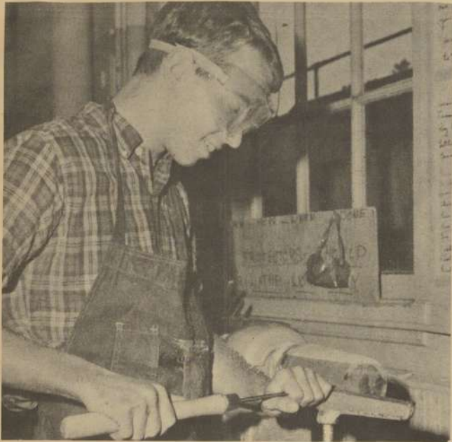
JUNIOR MIKE DUNN demonstrates the semi-finishing process involved in fashioning a wooden beer mug. Using a 'round-nose,' Mike carefully smooths the surface. While working on the lathe, goggles are worn to protect the eyes from flying fragments.
