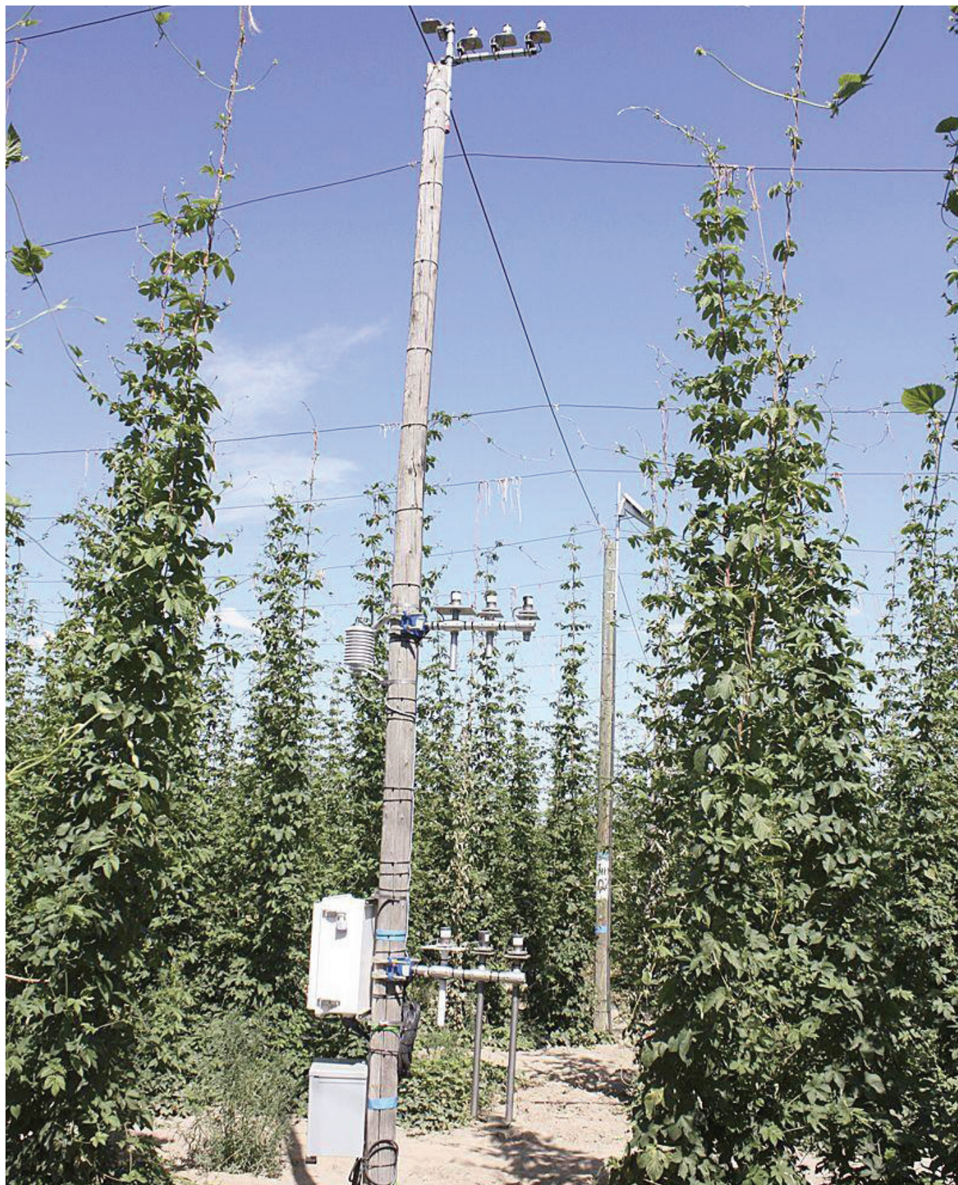
A Washington State University AgWeatherNet system monitors conditions in a hop yard.
