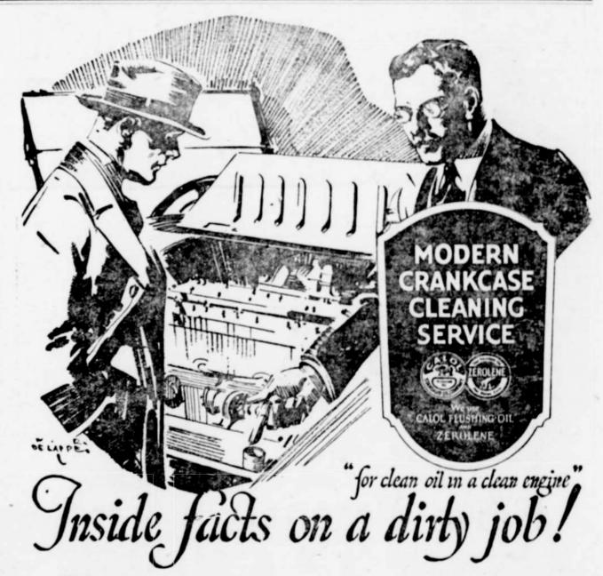
JOUR ENGINE requires an internal bath frequently, Road dust, carbon from the combustion chamber, and fine particles of metal worn from the bearing surfaces get into the lubricating oil in the crankcase. All this dirt circulates with the oil through the engine. If it isn't drained out regularly there's bound to be excessive wear and tear.
