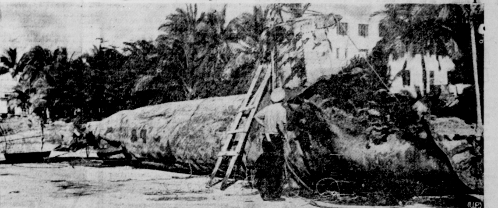
Hauled ashore, this two-man "sneak sub" is under study by U. S. Navy experts in Hawaii, where several subs of this type were used in attack on Pearl Harbor. This one was knocked out by shell through conning tower. It is believed to have range of only 200 miles and operates from mother ship. It packs two torpedoes and 300-pound demolition charge touched off by crew in suicide blast. (Passed by U. S. censor.)
