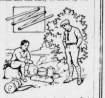
is shown in the drawing. made from a number of 18-in. lengths of 1/8-in. flat iron, about 1 in. wide. These lengths are pivoted together at the ends as shown in the upper detail, which arrangement permits them to be folded compactly or frawn out for use. The fire is made between two rows of rocks, as flat as can be found and of fairly equal height, as shown, and the grate placed on top of them. When not in use, the grate is folded up and put in a canvas pocket made to hold it.
