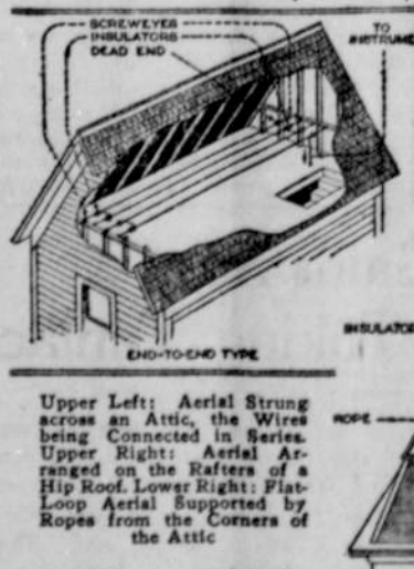
Upper Left: Aerial Strung across an Attic, the Wires being Connected in Series. Upper Right: Aerial Attached to the Rafters of a Hip Roof. Lower Right: Flat-Loop Aerial Supported by Ropes from the Corners of the Attic.
