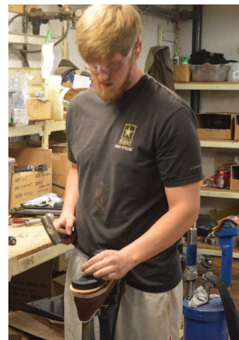
Above: Craftspeople at the Wesco factory in Scappoose build boots and shoes, cutting leather by hand and hand nailing the soles.
