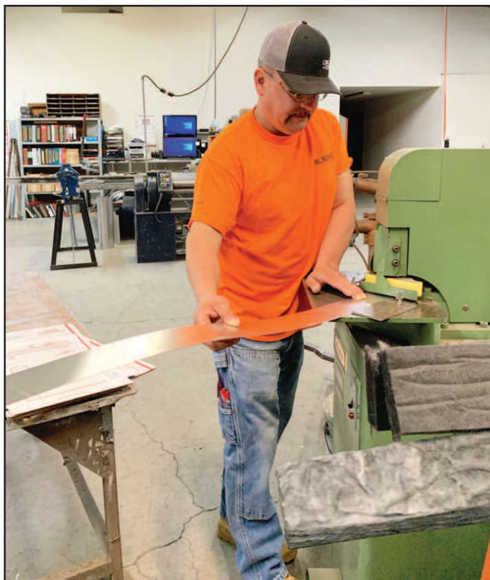
At Robert Lloyd Sheet Metal in Independence, Oregon, Sheet Metal Workers Local 16 member Robert Bettles shears a sheet of aluminum into strips to be used making facemasks to prevent the spread of COVID-19.
