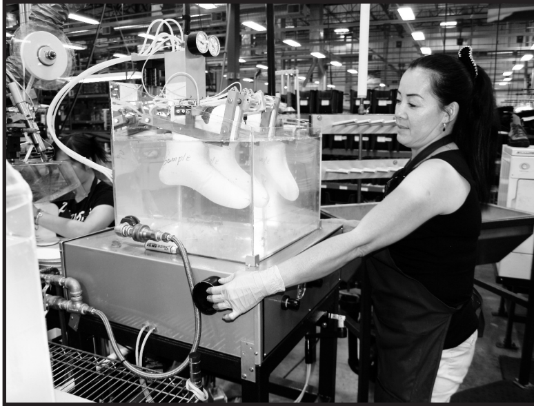
Bonavy Chum performs a water test on a GORE-TEX liner that goes in some styles of Danner Boots. UFCW members make Danner Boots at a 60,000 square-foot factory in Northeast Portland.
