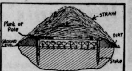
Fig. 1.—Cross Section of a Cabbage Storage Pen Made of Stakes and Poles and Covered With Straw—This is a Good Way to Store Cabbage.
